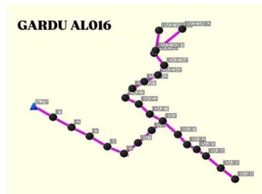
Gambar 3. Single Line Diagram JTR Gardu AL016 Sumber : PLN ULP Alas (2025)
