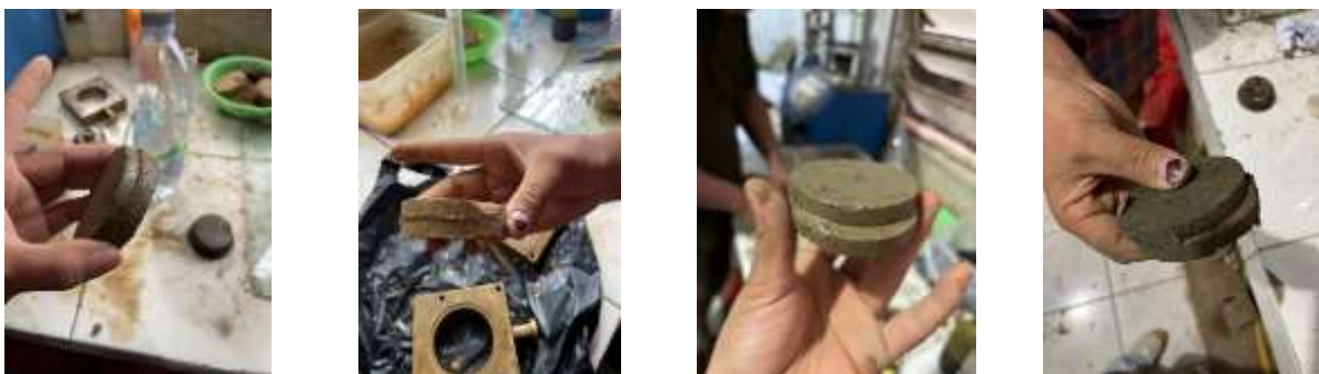
Gambar 3. Hasil Pengujian Kuat Geser Langsung Tanah Asli, 5%, 10%, 15%
