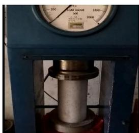
Gambar 8. Compression testing machine kapasitas 2000 KN
