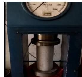
Gambar 7. Compression Testing Machine kapasitas 2000 KN
