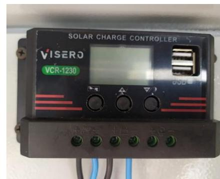
**Gambar 11. Solar Charge Controller**
